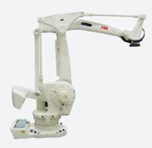
Introducing ABB's fastest palletizing robot, the ABB IRB 760. With a 450kg payload, this robot can move 60kg at 1500 cycles per hour or 450kg at 880 cycles per hour! This four axis robot is designed for faster, easier programming. The IRB 760 IRC5 uses ABB's QuickMove or TrueMove in order to allow for smooth & accurate production capabilities.
